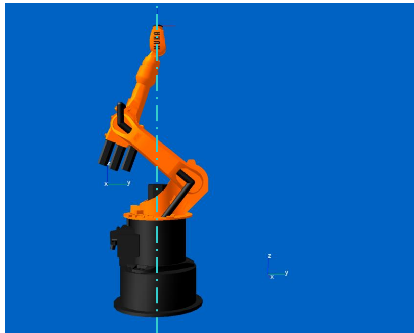
Figure 12: Robot in \alpha_1 -singularity
